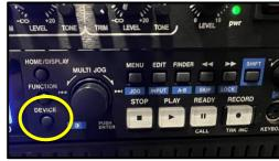
5. Press "Device" Button Choose the device you inserted in step #3 by pressing the "Device" button next to the large "Multi Jog" knob on the recorder.
