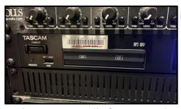
19. Remove Media from Recorder Once the Recorder finishes writing the files to your media device, you can remove your device from the recorder. Copy the files into a different location like your computer or OneDrive. If you checked out a USB Drive, be sure to return it.
