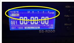
14. Check Audio Levels Check the Recorder Screen for proper audio levels. The audio meter should be peaking between 12 and 4. If it is not...
