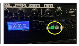
15. Press "Play" to Record To start recording, press "Play" on the Recorder. The Play button will light up green and the time will begin counting on the screen. If you need to pause the recording, press the Ready button. The recorder will go back to standby mode.
