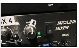
2. Ensure the Audio Mixer is on and Master Volume is up A green light should be on, and the switch flipped to the | symbol. The Master Volume knob should be turned to the arrow, as shown in the picture.
