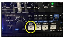
16. Press "Stop" to Stop Recording When you are done recording, or want to create a new track, press the "Stop" button. This will start to save your file to your media device.
