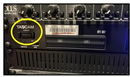
3. Ensure the Audio Recorder is on The screen should be on and blue. If it isn't, press the power button circled above.
